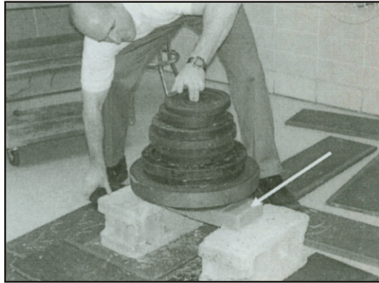
The bridge seen in this photo was made by sophomore Angela Smith and it held 347 pounds without breaking!
